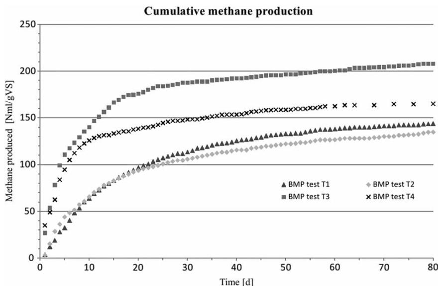
Figure 1. Cumulative methane production from BMP tests  $T_1 - T_4$ .
