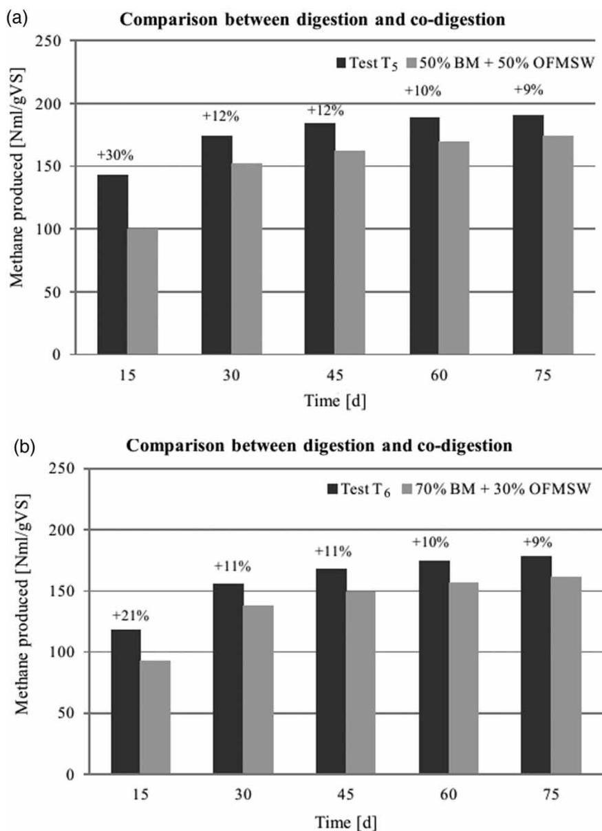
Figure 3. Comparison between digestion and co-digestion: (a) mixture with 50% BM and 50% OFMSW; (b) mixture with 70% BM and 30% OFMSW.
