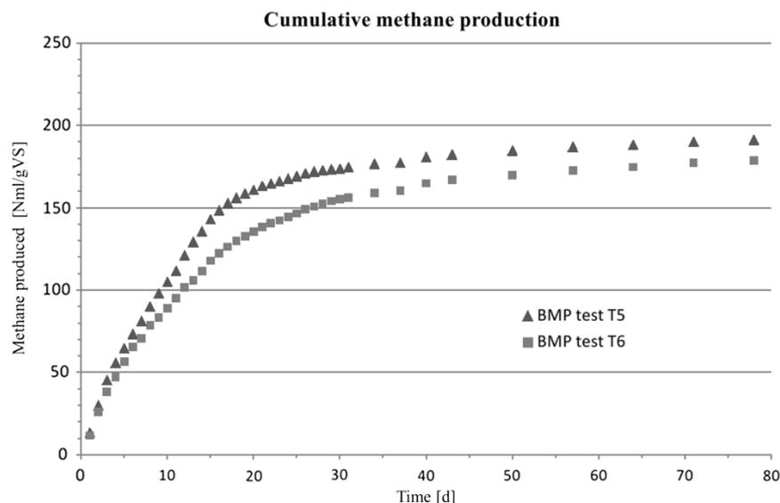
Figure 2. Cumulative methane production from BMP tests T<sub>5</sub> and T<sub>6</sub>.
