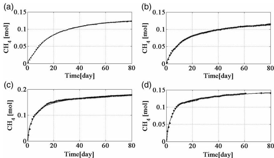
Figure 4. Comparison between experimental (points) and simulated (lines) methane production from BMP tests T<sub>1</sub> (a), T<sub>2</sub> (b), T<sub>3</sub> (c) and T<sub>4</sub> (d).
