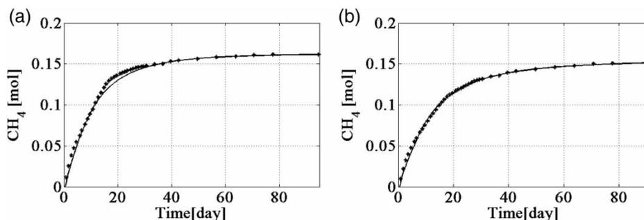
Figure 5. Comparison between the experimental (points) and simulated (line) methane production from BMP tests  $T_5$  (a),  $T_6$  (b).
