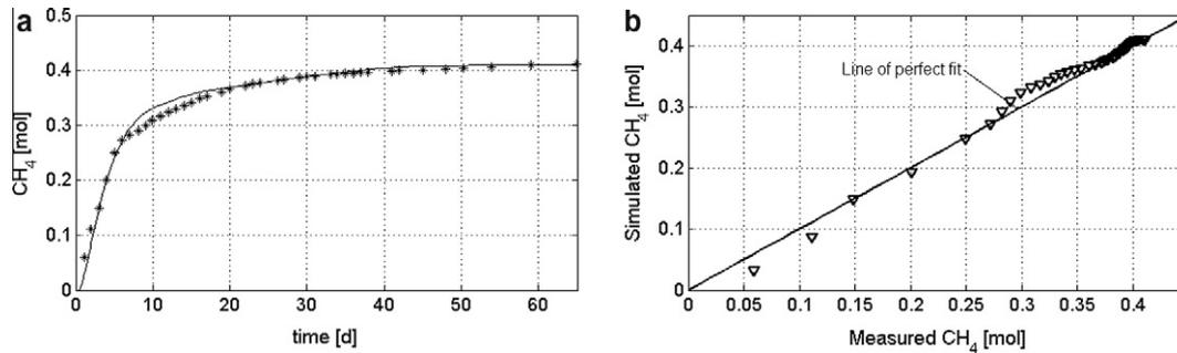
Fig. 7. Comparison of measured and simulated by proposed model cumulative methane production for experiments B: overlapping between measured and simulated data (a); comparison with the line of perfect fit (b).
