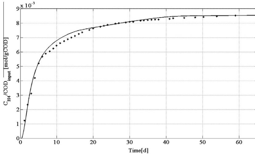
Fig. 9. Comparison of measured and simulated by ADM1 cumulative methane production for experiment B.
