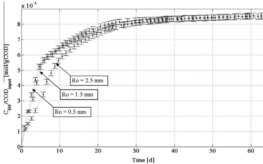
Fig. 2. Cumulative methane production obtained in the experimental tests A, B and C.
