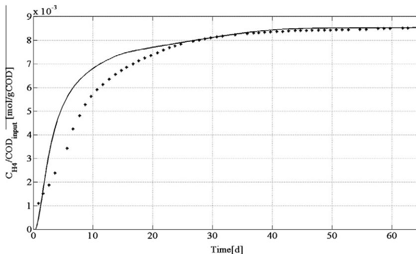
Fig. 10. Comparison of measured and simulated by ADM1 cumulative methane production for experiment C.
