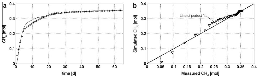
Fig. 6. Comparison of measured and simulated by proposed model cumulative methane production for experiments A: overlapping between measured and simulated data (a); comparison with the line of perfect fit (b).
