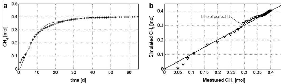
Fig. 8. Comparison of measured and simulated by proposed model cumulative methane production for experiments C: overlapping between measured and simulated data (a); comparison with the line of perfect fit (b).
