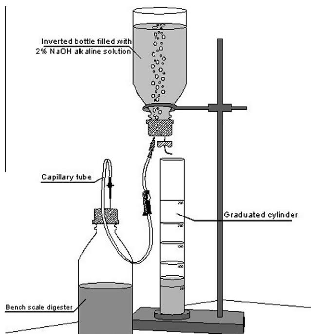
**Fig. 1.** Experimental equipment used to measure the daily methane production.
